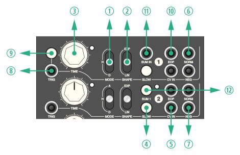
Figure 2: Control Elements of fourMative CONTOURS
