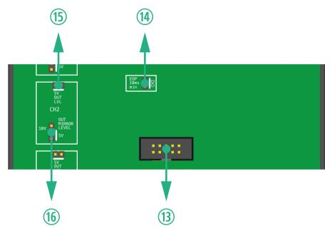
Figure 3: Jumpers and system-bus-connector of fourMative CONTOURS
