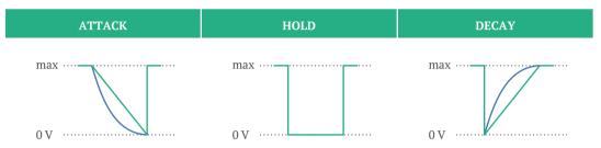
The voltage starts from its maximum, falls back to **0 V** with the adjusted envelope duration (**TIME** ③ / **CV IN** ⑤) and jumps back to its maximum upon completion.
