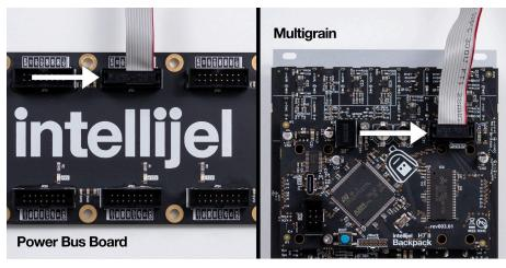
3. Connect the 16-pin end of the ribbon cable to an available header on your case's power bus board. Ensure the red stripe on the ribbon aligns with the side of the power header labelled "-12V" or similar marker. Current Intellijel cases use shrouded headers to help with orientation. If you're unsure, please check the manual for your power supply or case.
