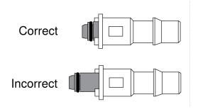
2. Insert the nozzle into the earphone, aligning the dots so it matches the keyed opening.
