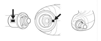
3. Place the threaded collar over the nozzle. After ensuring the threads are properly engaged, use the nozzle key to gently turn clockwise.
