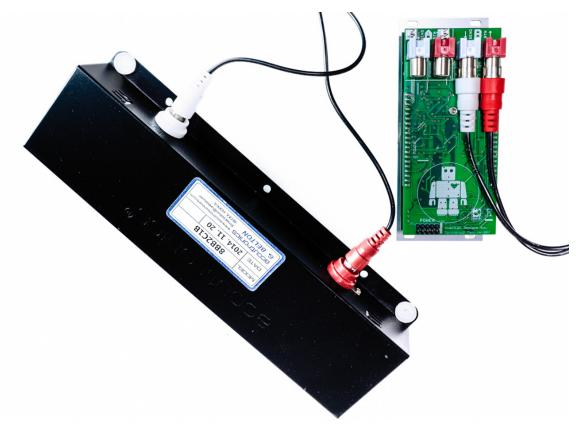
The smallest of the three Accutronics tanks does not come with an RCA connecting cable. Instead, it connects to the Springray<sup>2</sup> via two small, keyed connectors on the Springray<sup>2</sup> back panel **A** connector, as shown below:
