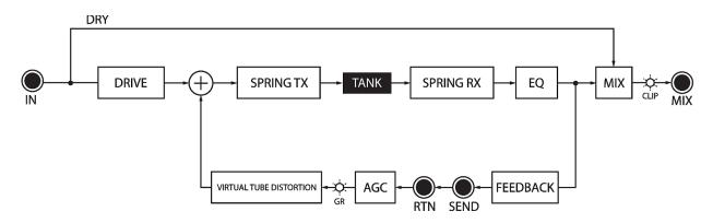
Springray<sup>2</sup> uses a feedback path with an asymmetrical FET-based **virtual tube distortion** circuit, which adds even-order harmonics for a pleasing overtone structure often associated with vacuum tubes.
