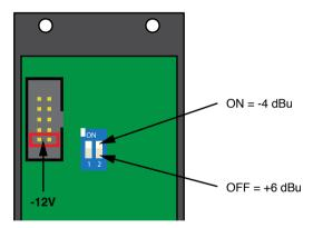
Figure 1: twinOUT rear with DIP switches and system bus connector
