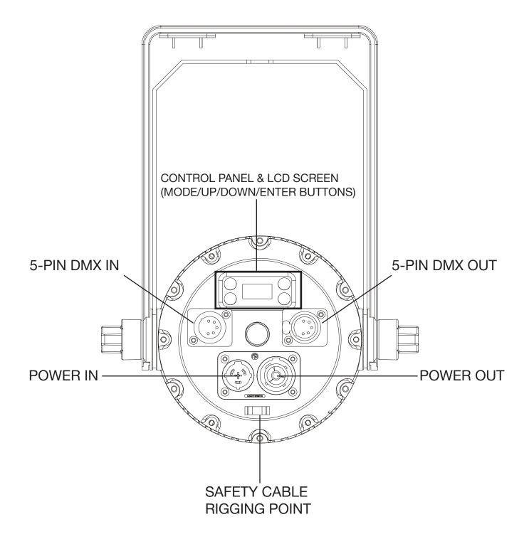
**DMX-512:** DMX is short for Digital Multiplex. This is a universal protocol used as a form of communication between intelligent fixtures and controllers. A DMX controller sends DMX data instructions from the controller to the fixture. DMX data is sent as serial data that travels from fixture to fixture via the DATA "IN" and DATA "OUT" XLR terminals located on all DMX fixtures (most controllers only have a DATA "OUT" terminal).
