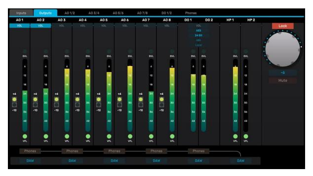
Line output level is switched between +4dBu and -10dBV nominal by the '+4/-10' radio buttons.
