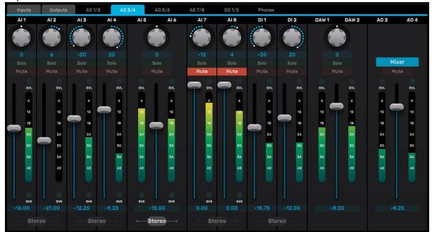
Each input channel has a fader, a high-resolution <u>peak meter</u>, with overload indication 0.05dB below clipping, plus mute and solo buttons and a pan-pot. By engaging the 'Stereo' button beneath an input pair, the pair is controlled by a single stereo fader, mute button and solo button, and the pan-pots are replaced by a single balance control. The DAW contribution and output strip are always in stereo mode.
