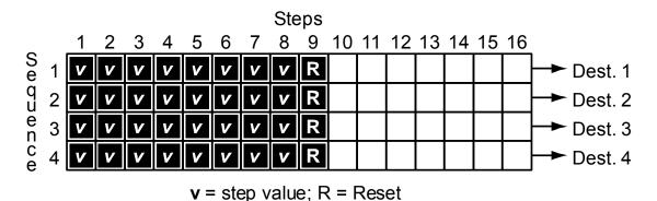
**Tip:** Using Reset while programming a sequence can be helpful. For example, when programming a specific melodic line, start by shortening the sequence to four or eight steps until those steps are set, and then gradually move the reset point to lengthen the loop until the desired number of steps is playing.
