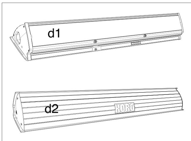
3. Lift the speaker box (d) by making the back side (d2) look toward you and the front side (d1) toward the Pa3X. Align its extruding guide (e) to the matching slot (f) on the back of the instrument (a). Slightly tilt the speaker box (d) forward, to prevent the fixing pin (k, *see below*) to damage the back of the instrument. To align them correctly, use one of the two plastic stoppers/delimiters (h) as a reference point, making one of the flanks or the speaker box's guide (e) touch it.
