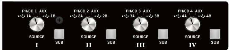
The same applies to USB port B. If your computer is connected to USB port B, switching a channel Source Select knob to USB B, assigns the corresponding virtual deck to that channel for audio playback.
