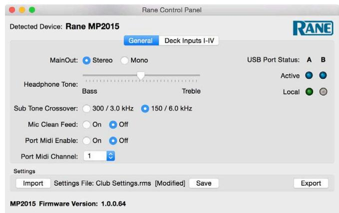
**Port MIDI Enable** enables MIDI commands to/from the MP2015 Mixer controls at the current USB Port. Default is Off.
