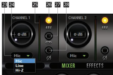
23. Mic, Line and Hi-Z (1, 2, 3, 4 only) modes selectable via dropdown menu (please ensure your selection from the dropdown menu matches the type of signal being inputted)
