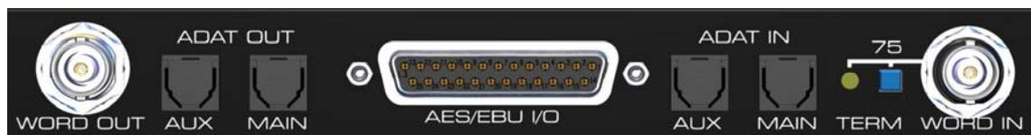
**WORD IN** (BNC): A push switch allows to activate internal termination (75 Ohms).
