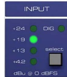
After selecting **DIG**, the digital input signal is routed to the digital outputs, with the AD-conversion being deactivated. The level meters now show the level of the digital input signal.
