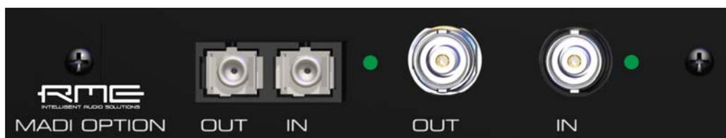
The MADi input will operate as an optional clock source (Clock section, OPTN) as well as a through input. Since each ADI-8 QS uses only 8 channels, up to 56 channels can be passed through.
