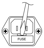
**3.** Remove the fuse and replace it with an equivalent-type fuse.
