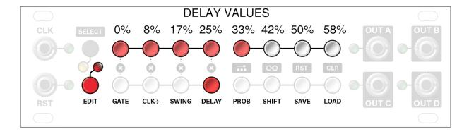
**NOTE**: If a track employs both a Delay and Swing (discussed above), those offsets will be summed. Gate lengths are maintained, however, if a step is swung and/or delayed so much that the requested gate length would overlap into the next step — then Steppy automatically shortens the gate to insure every step triggers.
