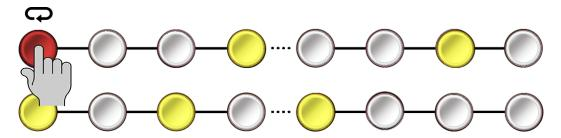
If Loopy (  $\infty$  ) is active, pressing two buttons loops playback between those steps, inclusive of the buttons you hold. So in the following example, Steps 1-4 loop for as long as you hold the buttons. Again, buttons outside the currently playing loop are **yellow** to indicate they are programmed into the pattern, but are not within the currently playing loop:
