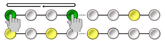
The standard Track position continues to advance normally as a loop plays. This means, when you release the buttons, the pattern reverts to playing exactly the step it would have played had you not looped a section.
