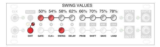
**NOTE**: If a track employs both a Swing amount and a Delay amount (discussed below), those delays will be summed. Gate lengths are maintained, however if a step is swung and/or delayed so much that the requested gate length would overlap into the next step, then Steppy automatically shortens the gate to insure every step triggers.
