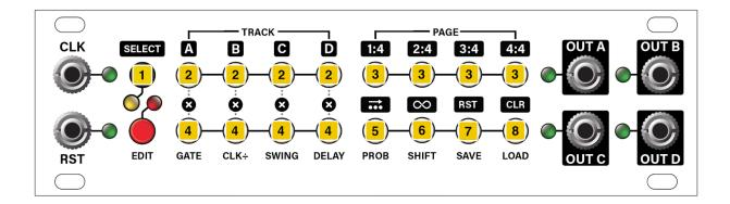
In Select Mode, the Multifunction buttons are used to select tracks for viewing & editing; to select pages within those tracks; and for enabling/disabling various track display and performance options.
