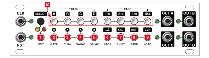
In Edit Mode, the Multifunction buttons select and modify various parameters (such as gate length, clock division, swing, etc.), as indicated by the labels beneath the bottom row of buttons. The red LED next to the EDIT button turns on when Edit Mode is on.
