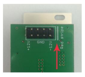
Most modules will come with the cable already connected but it is good to double check the orientation. Be aware that some modules may have headers that serve other purposes so ensure the cable is connected to the right one.
