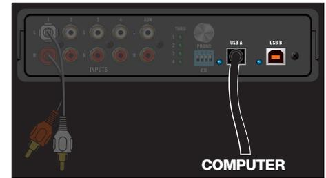
Using the provided USB cable, connect either USB A or USB B on your SL 4 to an available USB 2.0 port on your computer.
