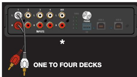
Connect your CD players or turntables to the SL4 INPUTS. If you use turntables, connect their ground wires to the ground terminal on either the SL4 or your mixer.
