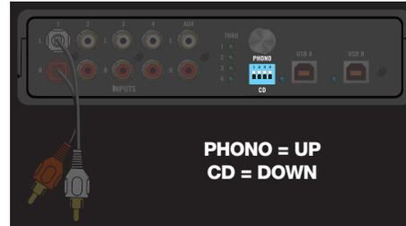
Set each input to the correct input level using the dip switches. Set the switches UP for Phono (turntables) or DOWN for CD players (line level).
