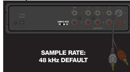
Use this to switch between 48 kHz and 96 kHz. Use 48 kHz by default if you are not using 96kHz audio files.
