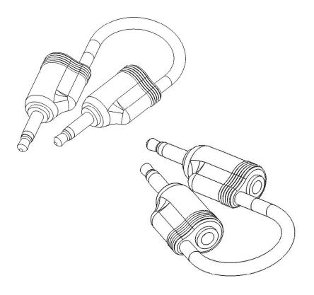
For the long operational life of the Stackcable do not pull it out using the cable. Doing so over time will destroy the internal connection, creating unstable signal flow and eventually resulting in the cables demise. Stackcablesshould only be pulled out using the molded head.
