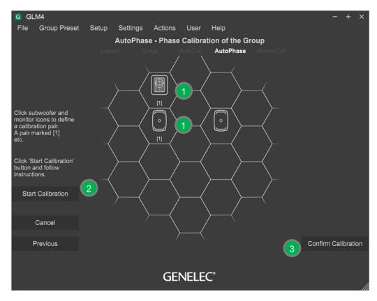
Figure 19. Steps in running the AutoPhase automatic phase calibration process
