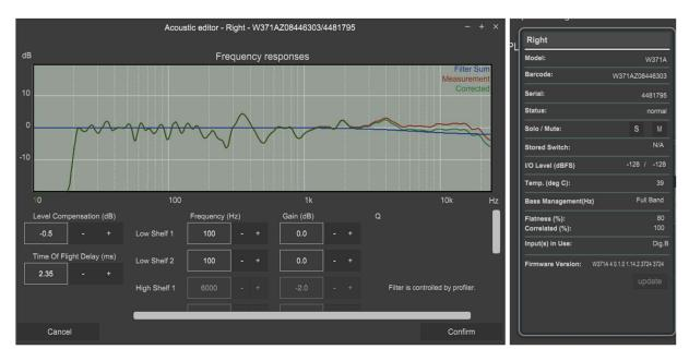
Figure 37. Acoustic editor for Woofer Systems and info on the Flatness and Correlation for Woofer Systems
