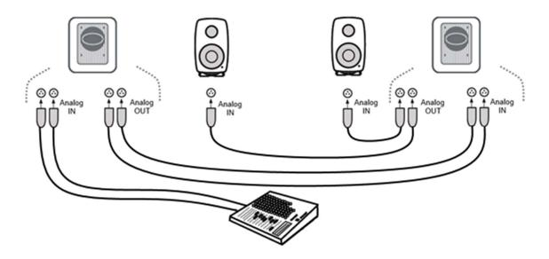
Figure 45. Dual subwoofers with the analogue signal.
