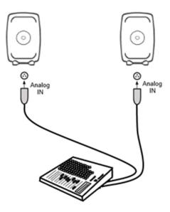
Figure 2. Analog stereo cabling.
