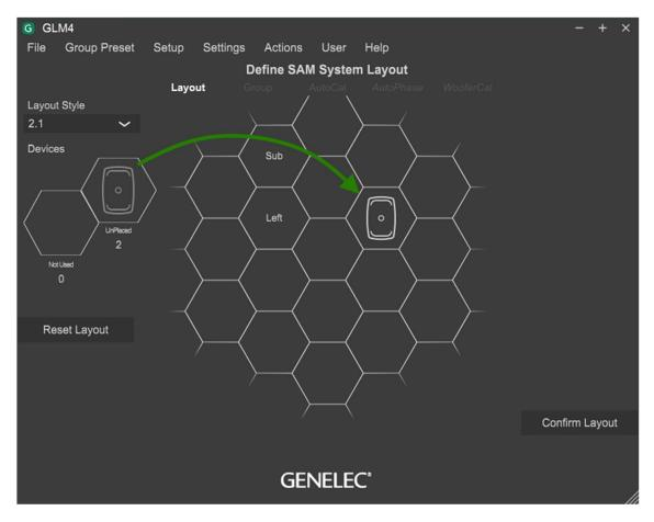
Figure 14. Drag and drop the monitor icons onto the layout grid to build a system layout
