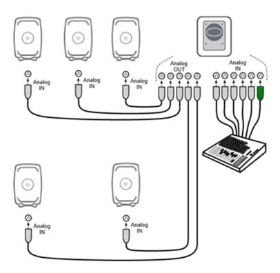
Figure 5. An example of analog 5.1 system cabling
