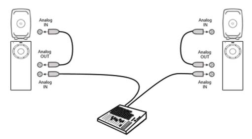
Figure 3. Analog stereo woofer system cabling.
