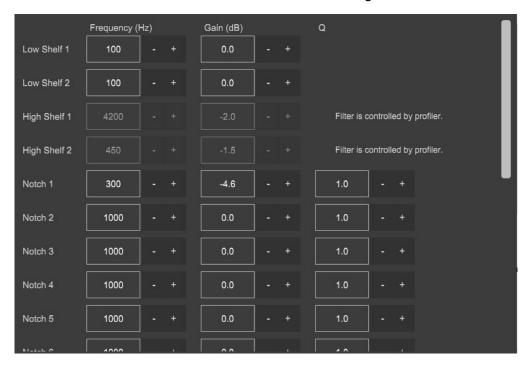
Figure 36. Room response equalizer controls
