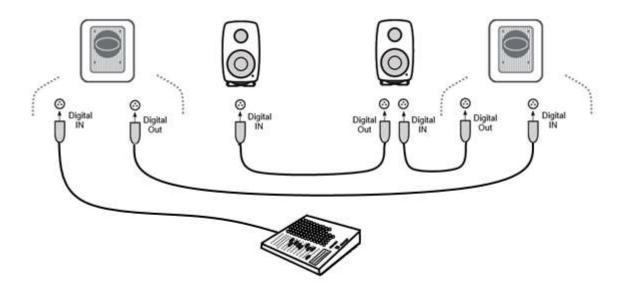
Figure 46. Dual subwoofers with the AES/EBU signal.
