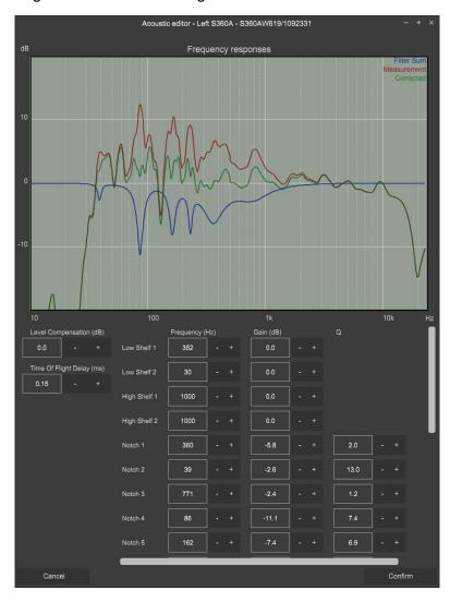
Figure 34. Example of the acoustical calibration editor window
