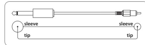
Fig. 5.2: Adapter cable with 1/4" jack
