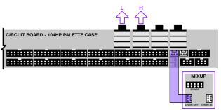
• **Mixup (IN)**: Connect the 3-wire link cable (provided with your Mixup module), between the Link Connector on the Palette circuit board and the CHAIN-IN connector on your Mixup.
