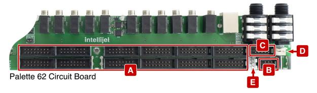
Running along the back edge of the Palette cases are their built-in circuit boards, which contain all of Palette's audio, midi, power, and module connection circuitry.
