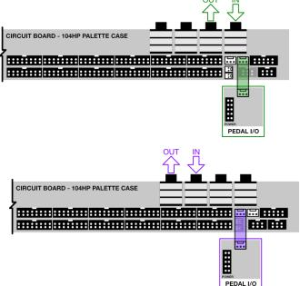
**IMPORTANT**: If you connect a module to the Links Connector, you should not connect a module to the same audio pair's Audio Jacks Connector (described previously), or unexpected results may occur.
