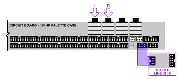
**IMPORTANT**: If you connect a module to the Audio Jacks Connector, you should not connect a module to the same audio pair's Link Connector (described later), or unexpected results may occur.
