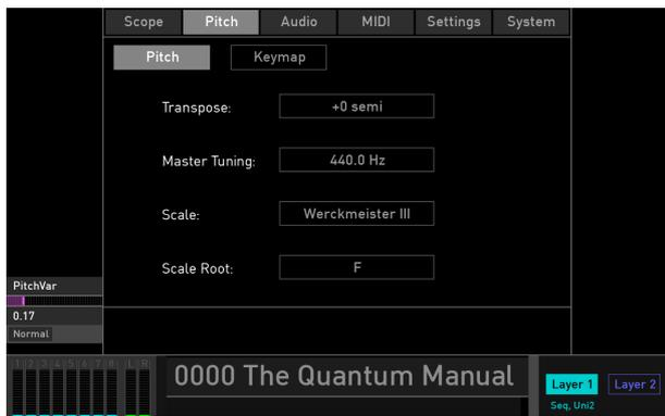
The **PitchVar** parameter (on the left display section) is global to all oscillators of all voices. It represents the **PitchVar** parameter that also can be found on the bottom of the Oscillator Control display page.
