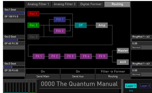
Here you will get a graphic overview of the Quantum's signal routing. You can also control the routing of the three oscillators, the ring modulators, and set up the audio outputs for the current sound.
