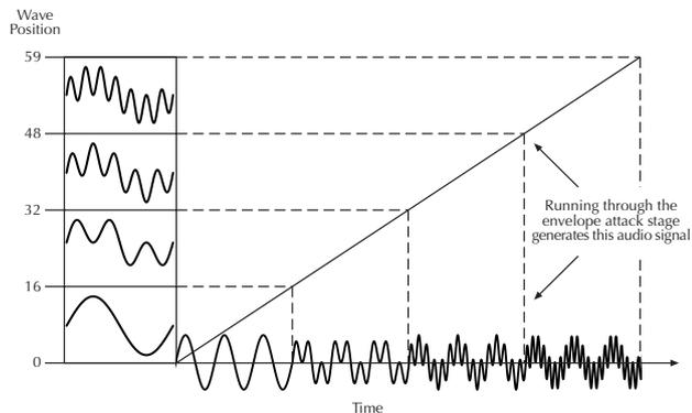
As soon as you play a note the envelope moves through the wavetable positions generating different waveforms over time.
