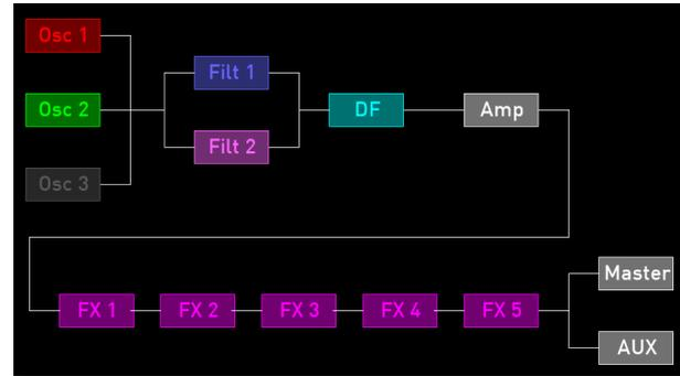
*Potential signal routing for an audio signal*
