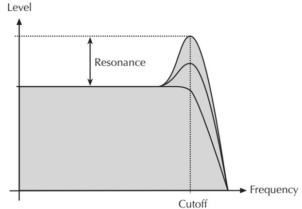
If the resonance is raised to a great extent then the filter will begin self-oscillation – i.e. the filter generates an audible sine wave even when it does not receive an incoming signal.
