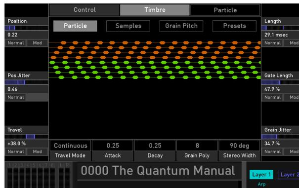
! The Particle parameter page can only be reached, if the Mode is set to 'Granular'. This can be done by tapping on the **Particles** button (and confirming the granular mode switch) or selecting *Granular* with the **Mode** parameter.
