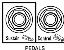
The **Control** Pedal input allows you to connect any suitable pedal. In the simplest case, you can plug in an expression pedal. For using its full-range signal as a modulation source the pedal needs to be calibrated using the “Control Pedal” button in Global->System->Calibrate.
