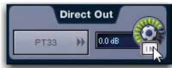
Activating a Direct Output on the Directs tab of the Patchbay
