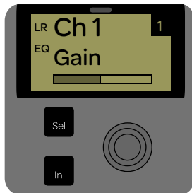
Channel display indicating the channel is selected
