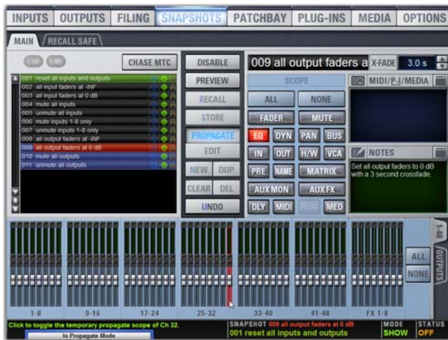
Propagating an EQ change for a channel
