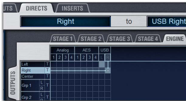
Assigning the Main Left-Right Direct Outputs to the USB recording inputs
