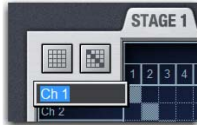
Naming and Input Channel from the Patchbay
