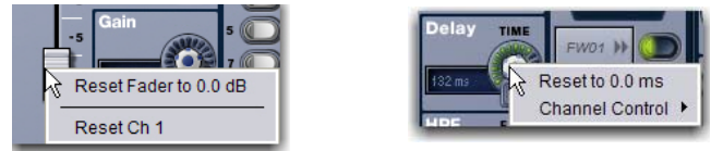
Right-clicking channel strip controls on-screen
