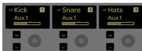
Channel encoders with Aux 1 sends assigned
