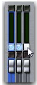
Unlinking a Mains fader
