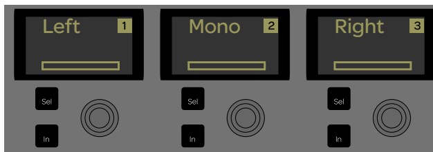
Channel displays showing Mains assigned to channel strips
