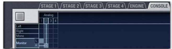
Assigning the Monitor bus to Console analog outputs
