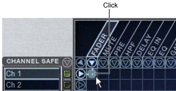
Enabling recall safe for channel 1 fader
