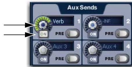
On-screen Aux send level control knob (top) and On button (bottom)
