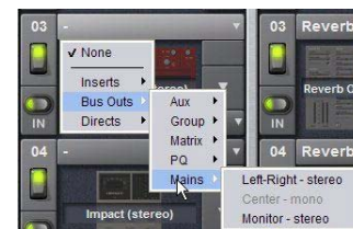
Assigning monitor output to a bus-fed plug-in
