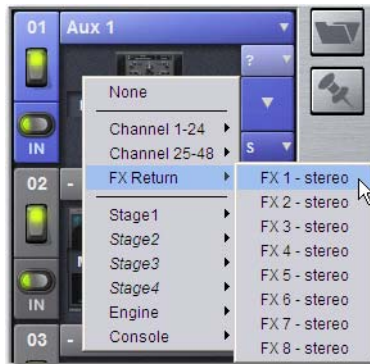
Assigning plug-in output to an FX Return
