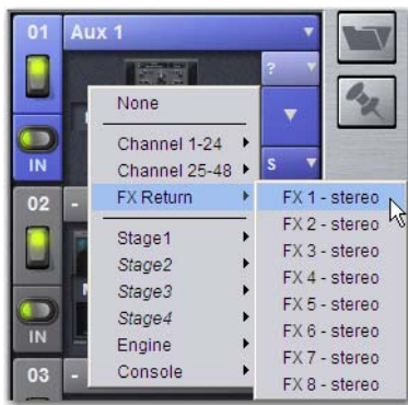
Assigning plug-in output to an FX Return
