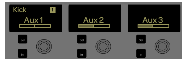
Channel Control with Auxes 1–8 assigned to Channel Control (Aux sends 1–3 shown)
