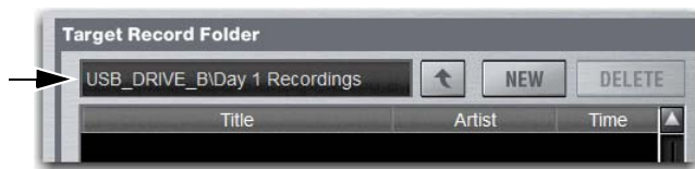
A folder targeted in the Target Record Folder section
