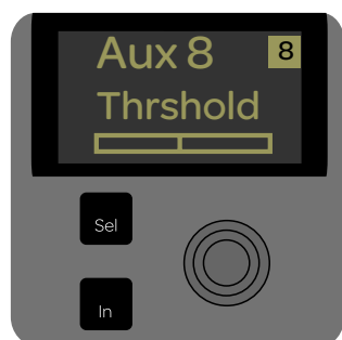
Comp/Lim Threshold assigned to a channel encoder
