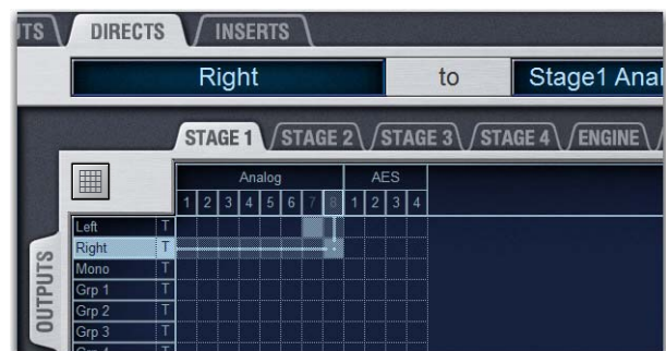
Assigning a Direct Output in the Patchbay
