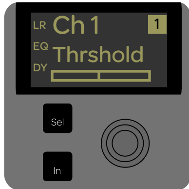
Comp/Lim Threshold assigned to channel encoders
