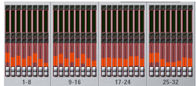
Snapshot channel fader display showing target fader positions
