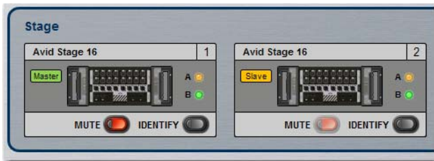
Assigned Stage 16s showing Master (left) and Slave (right) statuses on the Options > Devices page
