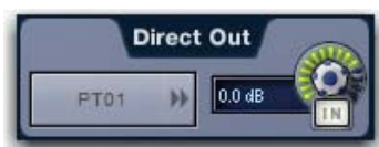
Direct Output controls in the Patchbay channel controls section
