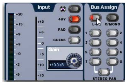
Assigning an input to the Mains Left-Right bus
