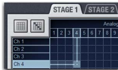
Assigning a hardware input to an Input Channel
