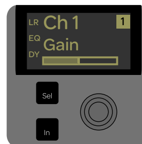
Gain assigned to the channel encoders
