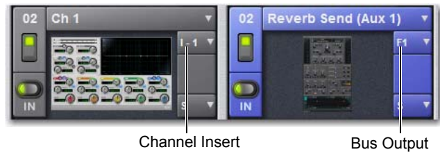
A mono plug-in inserted on a channel (at left) and a stereo plug-in assigned as a bus processor (at right)
