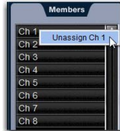
Removing an input assignments from a bus
