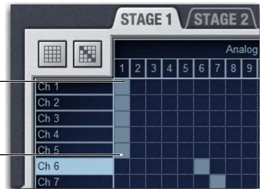
A hardware input routed to multiple Input Channels
