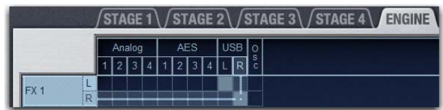
Assigning the USB playback outputs to an FX Return.
