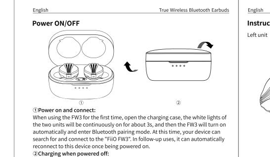
Put the two units into the charging case and close it. The FW3 will automatically
