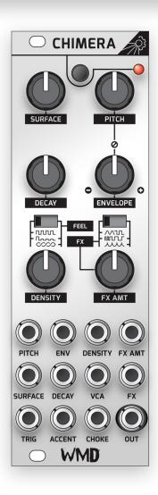
TRIG: Hit it with some pulses! For extra fun, trigger the module using the handy trigger BUTTON.
