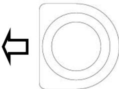
**Correct orientation of the power lead connector with the FLAT side facing Left**
