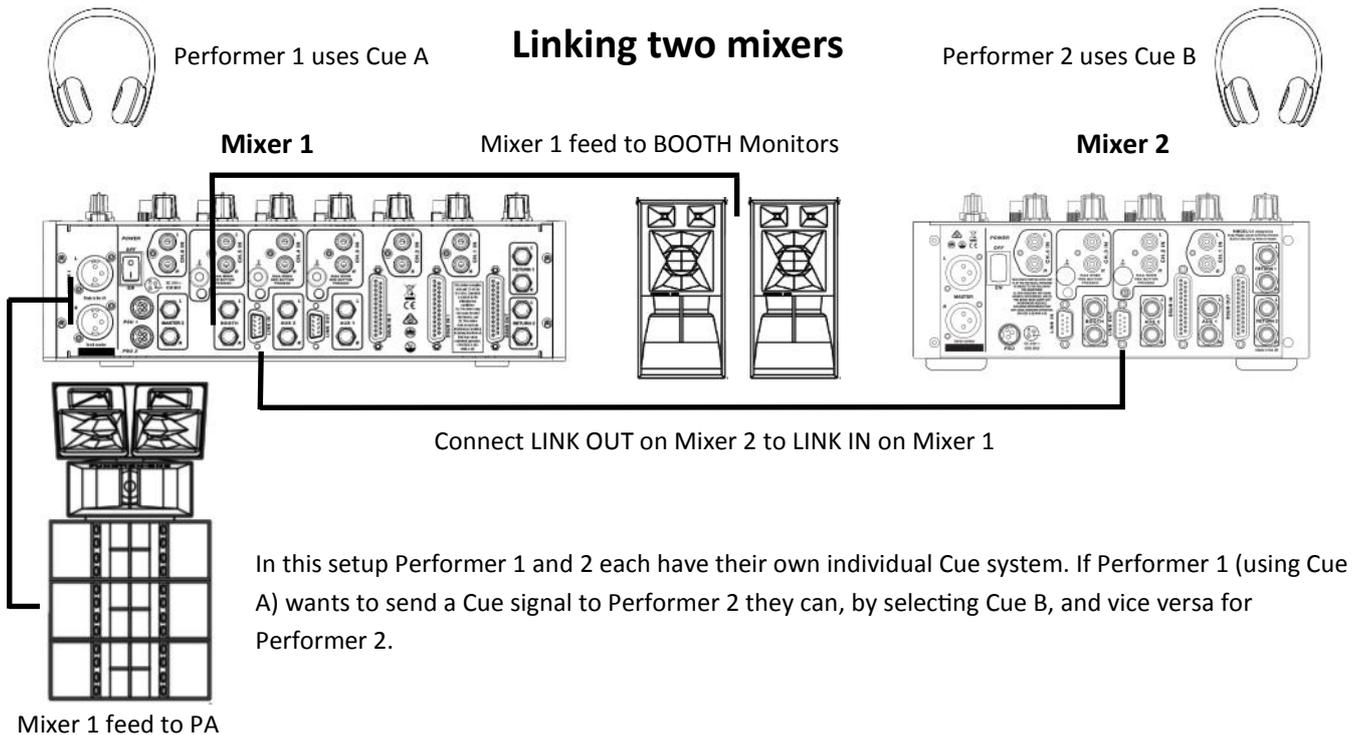
**IMPORTANT!** - When linking two mixers together, one will need to be assigned to feed its buss signal through the Link Cable and on to the main PA and Booth Monitor connected to the other mixer.
