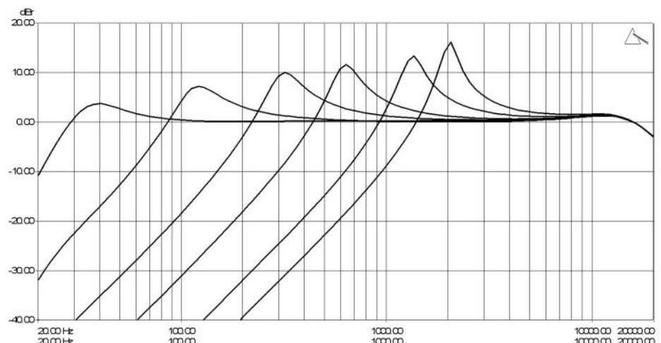
This graph illustrates how the resonance of the High-Pass Filter is automatically reduced as the frequency is lowered
