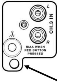
**RCA Inputs** - These are the default inputs to all four channels. On channels 2 and 3, the inputs can be configured for use with turntables by pressing the small red buttons located below each earth binding post. Channels that are configured for turntables (phono) will show the input selector switch illuminating red.
