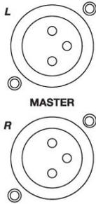
**MASTER** - Main mix outputs for direct connection to the system PA.
