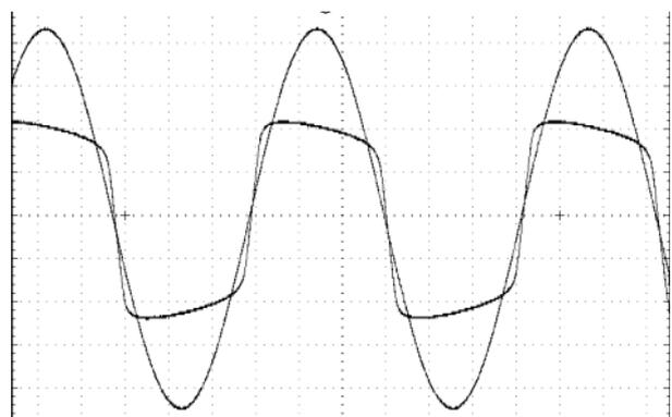
This shows the signal very heavily clipped, virtually to a square wave.
