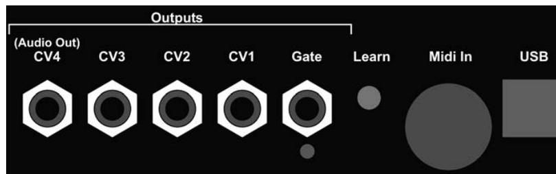
Depending on the incoming MIDI data (note on/off, notenummer, pitch bend, MIDI controller, velocity), the interface will generate:
