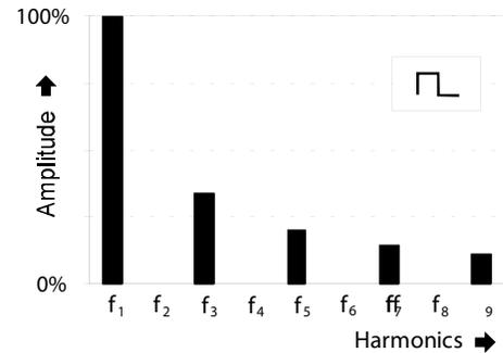
The **width of a pulse wave** can be modulated by a low frequency oscillator (LFO) or, less common, by an envelope generator. This way the harmonic spectrum of the pulse wave does not remain static. The resulting sound is similar to the chorusing effect between two oscillators which are nearly perfectly in tune, i. e. unison. The modulation frequency has to be very low (approx. 1 Hz or lower) because otherwise the oscillator will sound out of tune.
