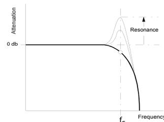
The resonance characteristics of a lowpass filter
