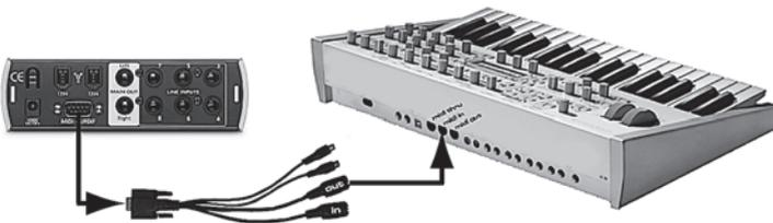
the breakout cable is securely connected to your FireStudio Mobile.
