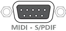
**MIDI and S/PDIF Breakout-Cable Connector.** This is where you connect the breakout cable for MIDI and S/PDIF I/O.
