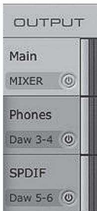
The FireStudio Mobile mixer has three output mixes, one for each of the FireStudio Mobile's three stereo outputs: mains, headphones, and S/PDIF.
