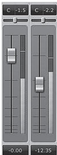
Move the channel fader up and down to increase and decrease the channel's audio level.
