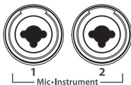
**Instrument Inputs** (Channels 1 and 2). The 1/4" TS connector on Channels 1 and 2 are for use with an instrument (guitar, bass, etc.). When an instrument is plugged into the 1/4" input, a high impedance input buffer is switched into the preamp circuit and the FireStudio Mobile becomes an active instrument preamplifier.
