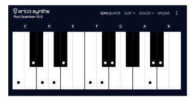
THE PICO QUANT PICO QUANT SCALE DESIGN INTERFACE ALLOWS YOU TO DESIGN YOUR OWN UNIQUE SCALES WITH 1/4 SEMITONE ACCURACY OR SELECT ONE OF 16 PREDEFINED SCALES. FOLLOW SIMPLE STEPS TO DESIGN AN UPLOAD SCALES TO THE MODULE!
