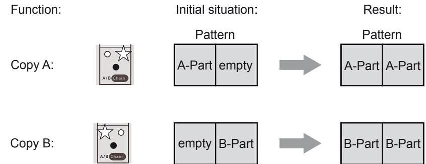
This is how to operate the Copy A / Copy B functions:
