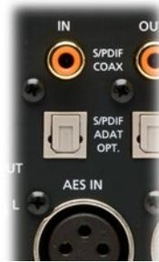
Hilo offers a choice of AES or S/PDIF as the digital input source. With S/PDIF you have the option of Coax or Optical Inputs.
