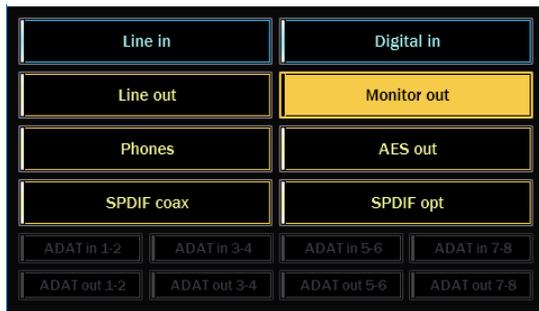
To select the meter source, press into the Source Select button below the Meters and select the desired source. Inactive sources will be grayed out.
