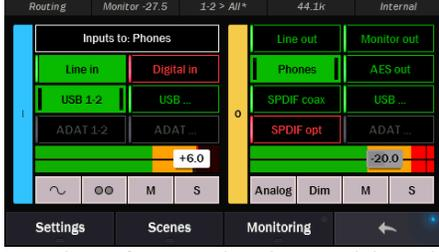
This performer likes the levels of the backing tracks louder, but the overall level down a bit, so we’ll nudge the USB Play source signal up by 6dB, and attenuate the Phones output by 10dB.
