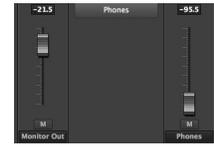
The source selection buttons allow the RTA to be used for any input or output on the Hilo. The faders allow analog volume control for the Monitor or Phones.
