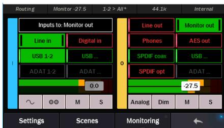
We already have signal from USB Play 1&2 carrying the streams from the computer. Now let’s add Line In as a source so there is the new guitar parts along with the existing tracks. We also set Monitor out at -27.5 as a good listening level.
