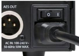
If all items are present, connect the Hilo AC power cord to a grounded AC Outlet, or power distribution unit. Switch on the power switch on the back of Hilo (note: the “|” position on the power button is “On” and the “O” is “Off”).
