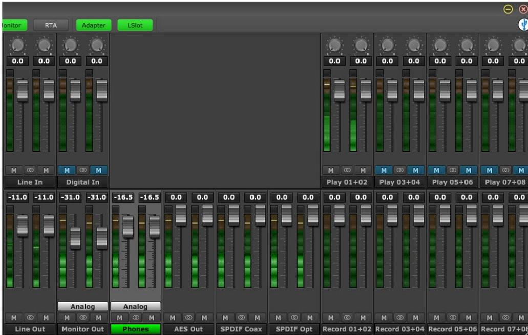
The Monitor page is where signals are routed, levels and pan settings are established, and meters can be viewed for all channels on the Hilo. It is visible whenever the “Monitor” button is green in the Navigation Bar. The section on the right, with the Play and Record devices, is only visible when the LSLOT button is green.
