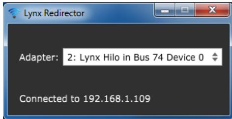
You should also see the “Connected to” indicator with the IP address of the Target Computer/Tablet show up on LynxRedirector on the Host Computer.
