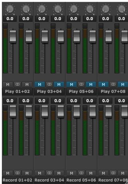
This button toggles whether controls for the LSLOT Sources are visible from the Main window or not. LSLOT sources are relative to the connection method used by the Hilo, USB, Thunderbolt or Dante record and play devices in the computer. This section will show the Play Sources (signals coming FROM the computer or Dante network) in the top row, and Record Sources (Signals going TO the computer or Dante network) in the bottom row.
