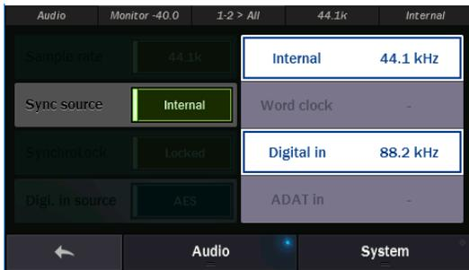
When you push the Sync Source button, you may select any of four possible sync options. If a clock source is valid, a sample rate will appear next to that selection. For instance, if a clock source is connected to the Hilo Digital input, next to “Digital in” there would appear the sample rate that the clock source is generating.
