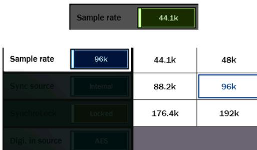
When Hilo is either clocked externally, or connected to the computer and subservient to the program or Operating System's rate (note: this is always the case with a USB connection to the computer), then the Sample Rate field is for display purposes only and is “grayed out”.
