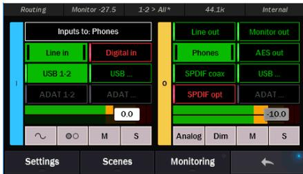
Now we’ll add Line In, so the performer can hear their input signal. Again, we’ll set the Monitoring Mode to “left” so their input signal is panned center in the headphones.
