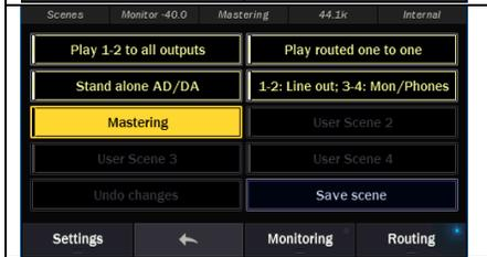
The new scene will now appear in the list, and will also appear as the active scene from the status strip. Scenes save volume position for outputs and sources, so keep in mind that there may be a change in level when a scene is recalled. Adjust monitoring equipment appropriately.
