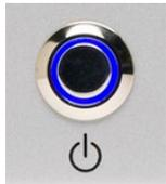
Hilo may power up automatically when AC is applied (this varies by firmware version). If not, press the front panel standby switch and verify that Hilo powers up.
