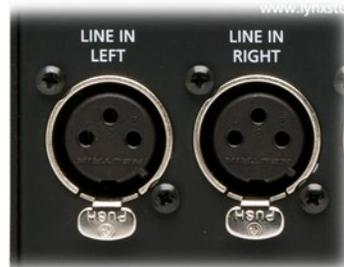
Line in trim can be set to any of eight preset trim settings. The Line in trim button shows the currently selected trim level, it is the same for the Left and Right inputs.
