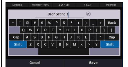
An onscreen keyboard will appear for inputting the scene name. Click the “x” at the end of name field to delete the factory name, if desired.
