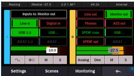
The guitar level is a bit hot compared to the mix. Let’s attenuate the Line In signal by 10dB.
