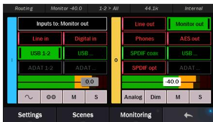
Let’s start by setting levels for the recording engineer. Start by selecting “Monitor Out” as the active Output:
