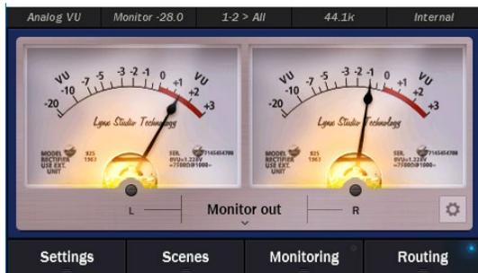
The Analog VU was designed in house to be as accurate to a true VU meter as possible. A single stereo input or output source can be selected at a time.
