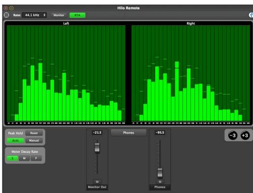
Monitor view will be explored in depth in the section below. RTA view presents the user with a high resolution Analysis Tool. This is an expanded version of the RTA that is available for the Hilo touchscreen display.
