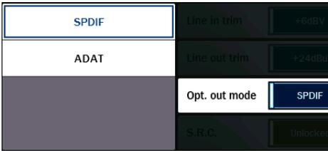
Hilo's Optical inputs and outputs can be used for either stereo SPDIF operation, or 8 channel ADAT operation (at 48 kHz). Hilo also supports the S/MUX protocol for ADAT Light pipe operation at higher sample rates. The ADAT Ports support 4-channels at sample rates of 88.2/96 kHz. Sample rates of 176.4/192kHz are not supported for ADAT S/MUX.
