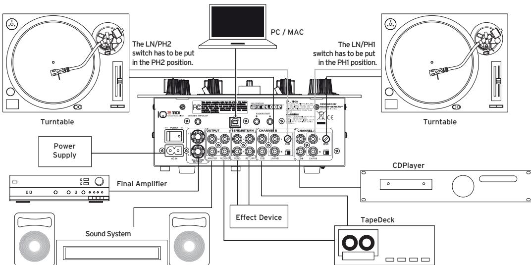
The Reloop IQ2 MIDI disposes of an integrated professional audio interface with 24 bit/96 kHz. Therefore a further external or integrated PC soundcard is not necessary. In the following you can find a list of possible connections:
