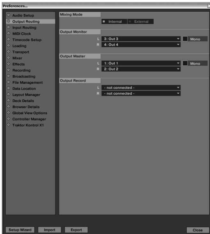
Put the IQ2 MIDI's Channel Signal Input Selector -6- channel A to the "MIDI1" position and channel B to the "MIDI2" position. This way the complete channels A+B are active in MIDI mode. This means Gain, 3-band EQ and linefaders do not influence the audio signal. They will just send MIDI messages. This mode is for users who would like to use the Traktor software mixer.
