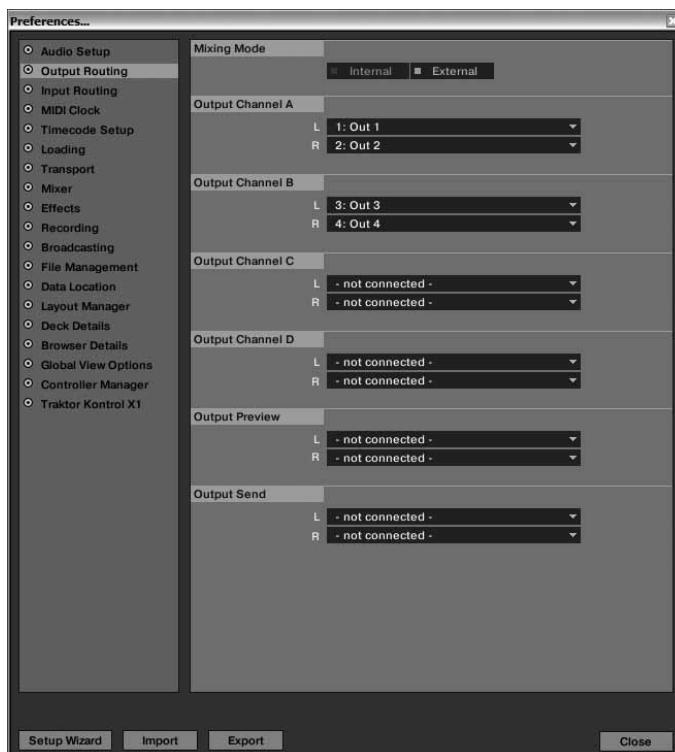
Put the IQ2 MIDI's Channel Signal Input Selector -6- channel A to the USB1 position and channel B to the USB2 position. This way the virtual Traktor channels will be routed to the mixer's hardware channels.
