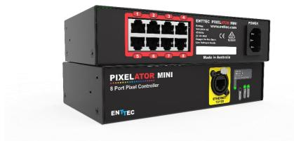
ENTTEC'S PIXELATOR MINI is an 8-port Ethernet pixel controller. Using ENTTEC'S PLINK protocol, each port provides data to ENTTEC'S PLINK INJECTOR which can control up to 2 Universes each, making the PIXELATOR MINI powerful enough to control up to 8,192 channels (2,730 RGB Pixels) with perfect synchronization across all eight of its outputs.
