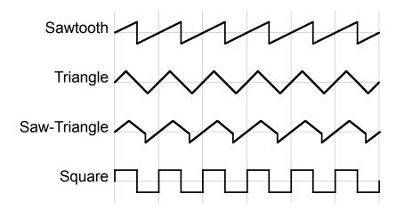
**Pulse Width:** 0...99—Sets the pulse width or *duty cycle* of the square wave. A value of 50 results in a true square wave with equal alternating high and low levels. Increasing or decreasing the value from 50 causes the waveshape to become asymetrical. Lower values narrow the postive-going portion of the
