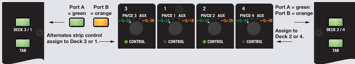
For control of opposing decks, the center channels of the Sixty-Four are wired to Decks 1 and 2, and the outside channels are wired to 3 and 4. This places pairs of decks centered over the crossfader.
