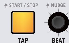
The effect time is normally a product of the BPM and the Beat Multiplier. If the right arrow ► or left arrow ◀ appears, there is an inequality between the BPM\*Beat and Time. The arrow indicates which way to adjust the Beat Multiplier to correct the inequality and get the closest possible time. If the BPM source is displayed (\*, S, A, B), the BPM\*Beat matches the displayed Time.
