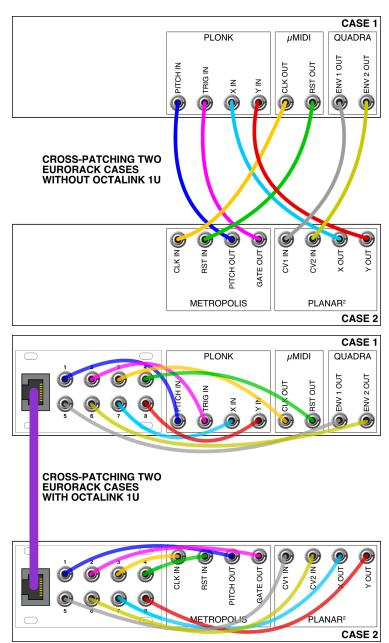
cable. Make sure to use only shielded Cat-6a or Cat-7 RJ45 cables. In general, you can spot a shielded cable by the presence of a metal-wrapped connector.
