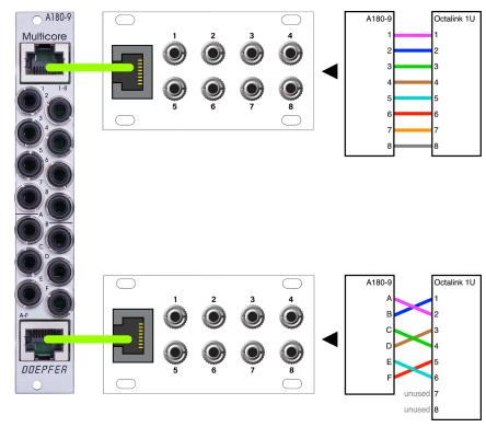
Note, in this illustration, the criss-cross manner in which numbered Octalink 1U jacks map to the lettered ports on the A-180-9.
