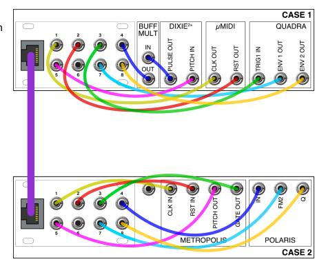
cables). Because the output of the  $Dixie^{2+}$  is an audio signal, we have chosen to first patch it through a Buff Mult on its way into the CASE 1 Octalink.
