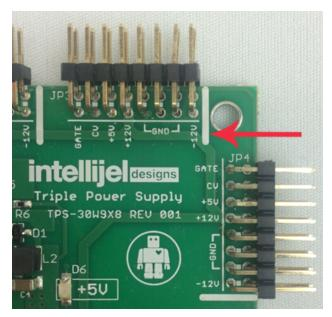
The other end of the cable, with a 16-pin connector, connects to the power bus board of your Eurorack case. Ensure the red stripe on the cable lines up with the -12V pins on the bus board. On Intellijel power supplies the pins are labelled with the label "-12V" and a thick white stripe:
