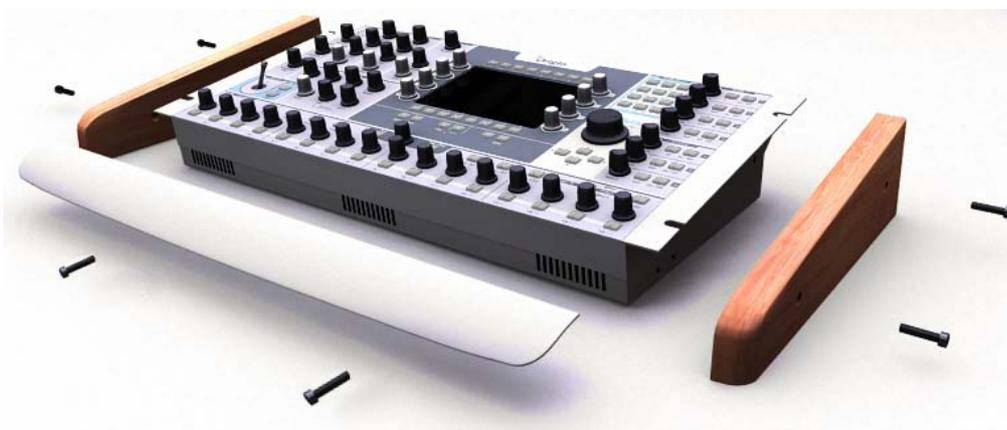
*Unscrew the two wood sides and the hand rest*
