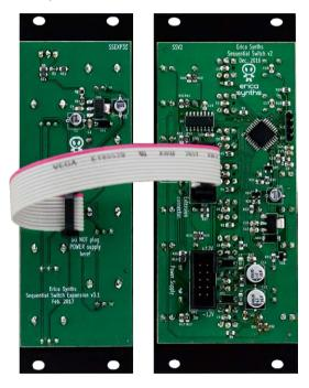
**SEQUENTIAL SWITCH CV EXPANDER** is connected to the Sequential Switch via IN/OUT jack switching lugs, which means, if you patch something into IN/OUT jack, the relevant input gets disconnected from the CV Expander.
