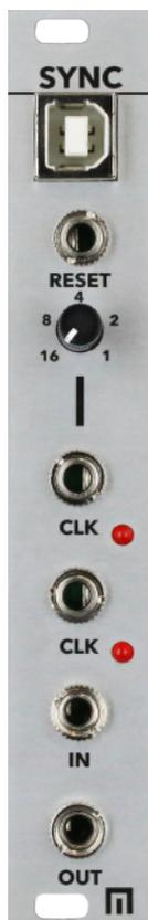
1. Make sure your case is powered up and that SYNC is connected to your computer via USB. It is recommended to connect directly without using a usb hub.
