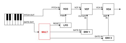
Since such a patch requires that one signal (a gate, in this case) be routed to three destinations, you need some sort of signal multiplier to accomplish this.
