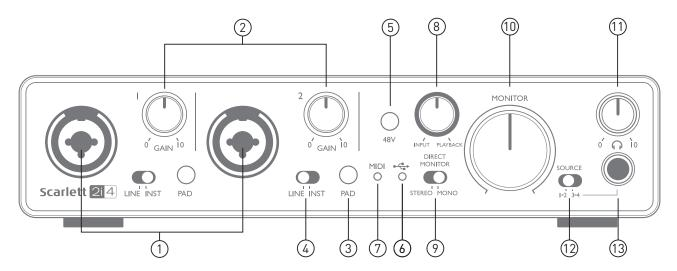
The Front Panel includes the input connectors for Mic, Line and Instrument signals, as well as the input gain and monitoring controls.
