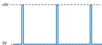
**Figure 9: Typical Gate Signal**
