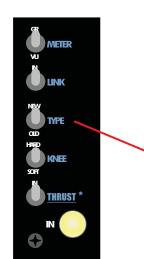
The 527 Compressor can be set to operate in two circuit topologies:
