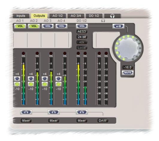
Line output level is switched between +4dBu and -10dBV nominal by the '+4/-10' radio buttons.
