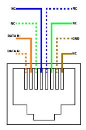
Plink Punch down pinout
