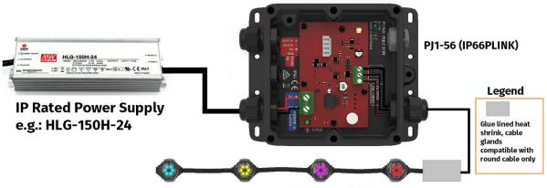
9PDOT1 IP67 rated RGB 24V pixel dots
