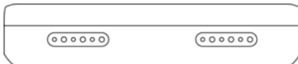
Control Blocks each feature 4 DNA connectors. These six-pin connectors magnetically connect multiple Blocks and also transmit power and data between the Blocks.
