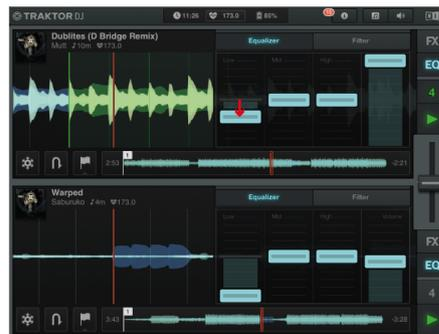
The LOW EQ of Channel A being turned anti clockwise and the corresponding affect in TRAKTOR DJ's Equalizer.
