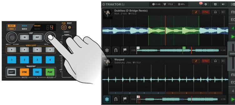
Triggering a loop in TRAKTOR DJ using the Loop Encoder.
