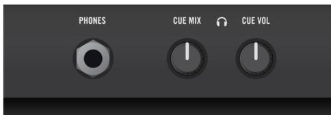
The Headphones input and CUE controls on the front panel of the S4.
