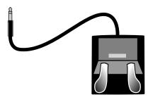
The SW1 (SUSTAIN) and SW2 jacks can be connected to dual switch pedals (2 pedals per jack), allowing up to four switch pedals to be used. Compatible pedals should use a single 1/4 inch tip-ring-sleeve (TRS) plug. (Two single switch pedals can also be plugged into one jack by using a 1/4 inch stereo (male) to dual mono (female) cable, aka TRS male to dual TS female.)
