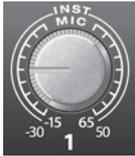
**Input Gain/Trim Control.** These knobs provide the following gain structure:
