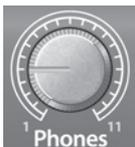
**Phones.** The Phones knob controls the volume of the headphone output on the front of the unit. The headphone amplifier is quite powerful, and the volume goes to 11, so use the maximum setting with extreme caution.
