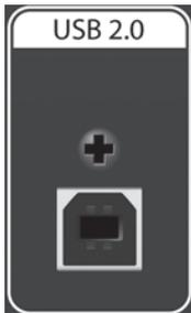
**USB 2.0 Port.** This is where you connect the USB cable from your AudioBox 22/44VSL to your computer. The AudioBox 22VSL is bus-powered via this connection and does not require an external power supply.
