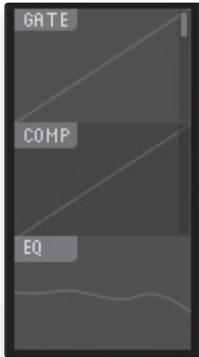
The AudioBox 22/44VSL provides a Fat Channel to process each input and DAW channel, the two effects buses, and the analog outputs in VSL. Each Fat Channel consists of a Downward Expander, a Compressor, a 3-band semi-parametric EQ and a Limiter. For more information on how these dynamics processors effect audio, please review Sections 5.2 and 5.3.
