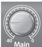
**Main.** The Main knob controls the output level for the Main Outputs on the back of the AudioBox, with a range of -80 dB to 0 dB.
