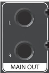
**Main Out.** These are the main outputs for the AudioBox 22/44VSL. The output level of the Main Outs is controlled by the Main volume knob on the front of the unit.
