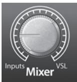
**Mixer.** The Mixer knob allows you to blend your input signals with the playback streams from your computer. This allows you to monitor your input signal with zero latency. If the knob is positioned at 12 o'clock, the input signal and the playback stream will be equally balanced. Turning the knob to the left will increase the level of the input signal relative to the playback stream; turning to the right will increase the level of the playback stream relative to the input signal.
