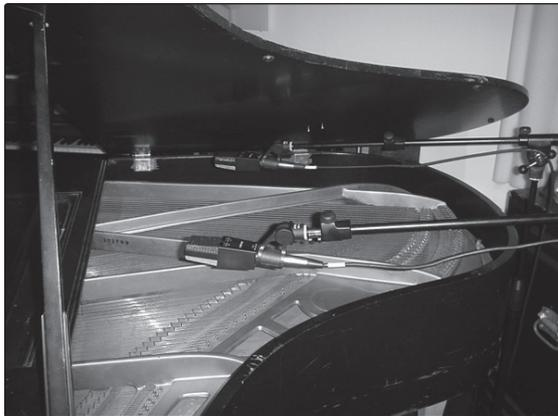
Place one microphone above the high strings and one microphone above the low strings. Experiment with distance (the farther back the more room you will capture). This technique can be used for live and studio applications.
