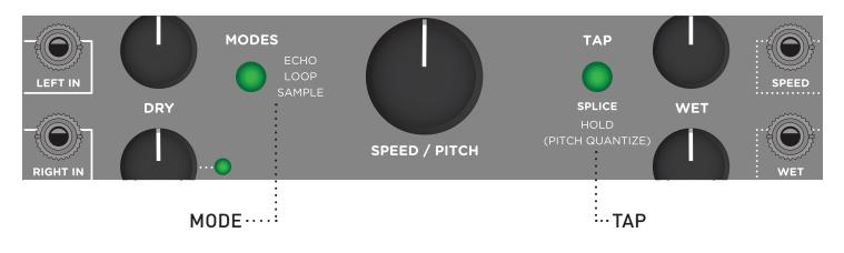
**SAMPLE mode: (RED LED)** Phrase sampler records an audio phrase between two taps of the TAP button. Transport **RESTART** (**I>**) triggers phrase playback.
