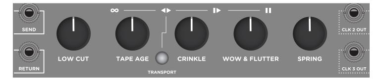
**LOW CUT:** Controls the low frequency shaping of the echo repeats. Set to minimum for extended low frequency bandwidth. Set to maximum for extremely high-passed, magnetic drum style repeats with a peaking response.
