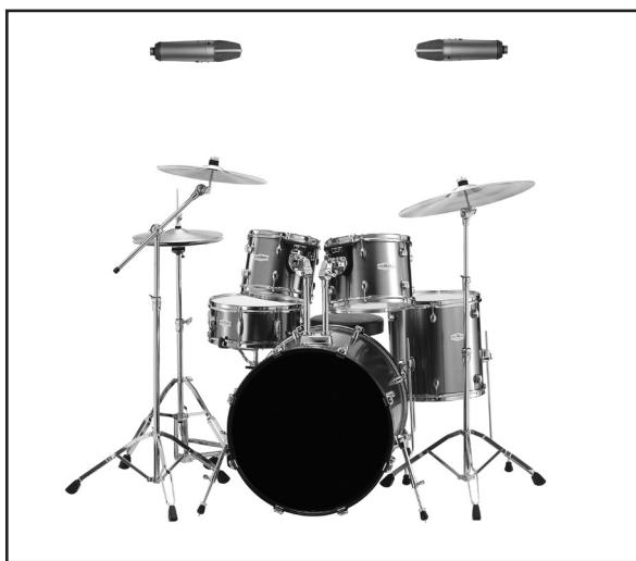
In this diagram, two WA-87's are used in a spaced pair configuration to record stereo drum overheads, maintaining equal distance from the snare drum for proper phase.
