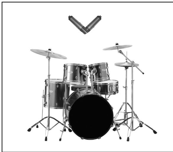
In this diagram, two WA-87's are used in a coincident pair, also known as XY configuration, to record stereo drum overheads.
